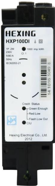
HXP100DI is a DIN Rail installation metering and control unit used in one phase two wire power network. Combined with CIU EV-KP or CIU EV-SP, it works as keypad or smart card split prepayment meter complying with STS standard.
