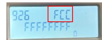
**\*Note:** If the CIU is still not communicating, it means that meter is in Cenelac-A frequency. So, the CIU also must be in the same frequency as the meter. Follow the steps to change the frequency.
